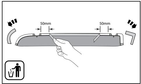
4. Angle the clips downward, align the cutouts with the clips and slide the Visor (3) into the door glass seal in front of the clip.
