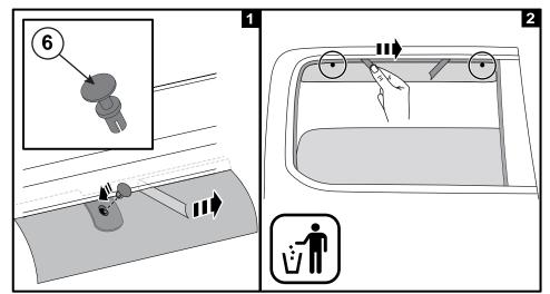
6. Pull the bottom outwards while raising and lowering the window a minimum of 5 times.
